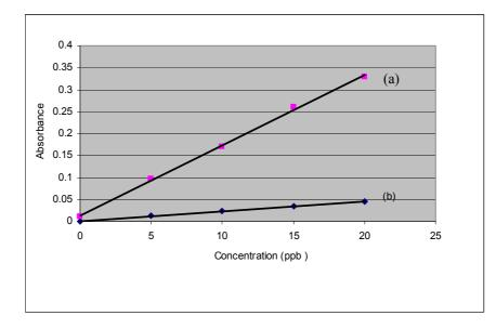
Fig. 1 Concentration versus absorbance curves for (a) chromium and (b) copper.
